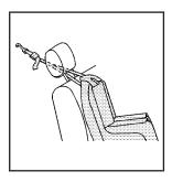
If the position you are using has an adjustable head restraint and you are using a dual tether route the tether under the head restraint and in between the head restraint posts. See Head Restraints on page 15.
